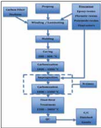
Fig 4: Flow Chart for the Manufacturing of Carbon/Carbon Composite Material
