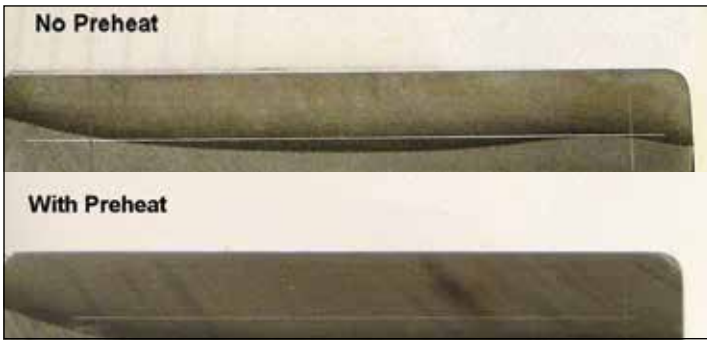
Figure 1: Macroetched cross-section showing differences in induction hardened case depth due to a 350°F preheat. All process parameters were the same for each trial. Horizontal line is at 7 mm inch depth. [10% Nitric acid etchant]
