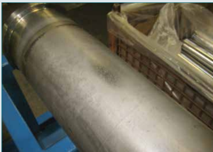
Fig. 1: A polished surface after acid etching shows an induction case termination at top left.
