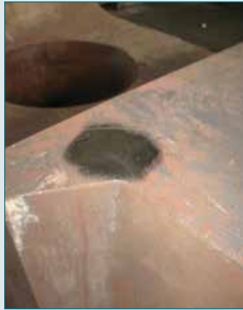
Fig. 4: Light grinding and polishing is needed for hardness testing of a large "one of a kind" casting.
