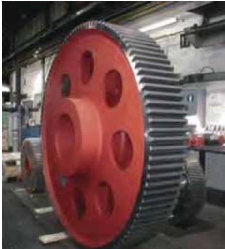
Figure 13: Rim materials, e.g., 18CrNiMo7-6, hub and rim materials e.g., C35, C45, 34CrMo4, 42CrMo4, 36CrNiMo8
