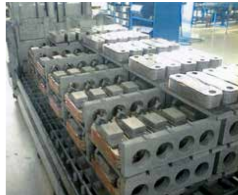
Fig 2: Load of Heat Exchangers for Brazing
