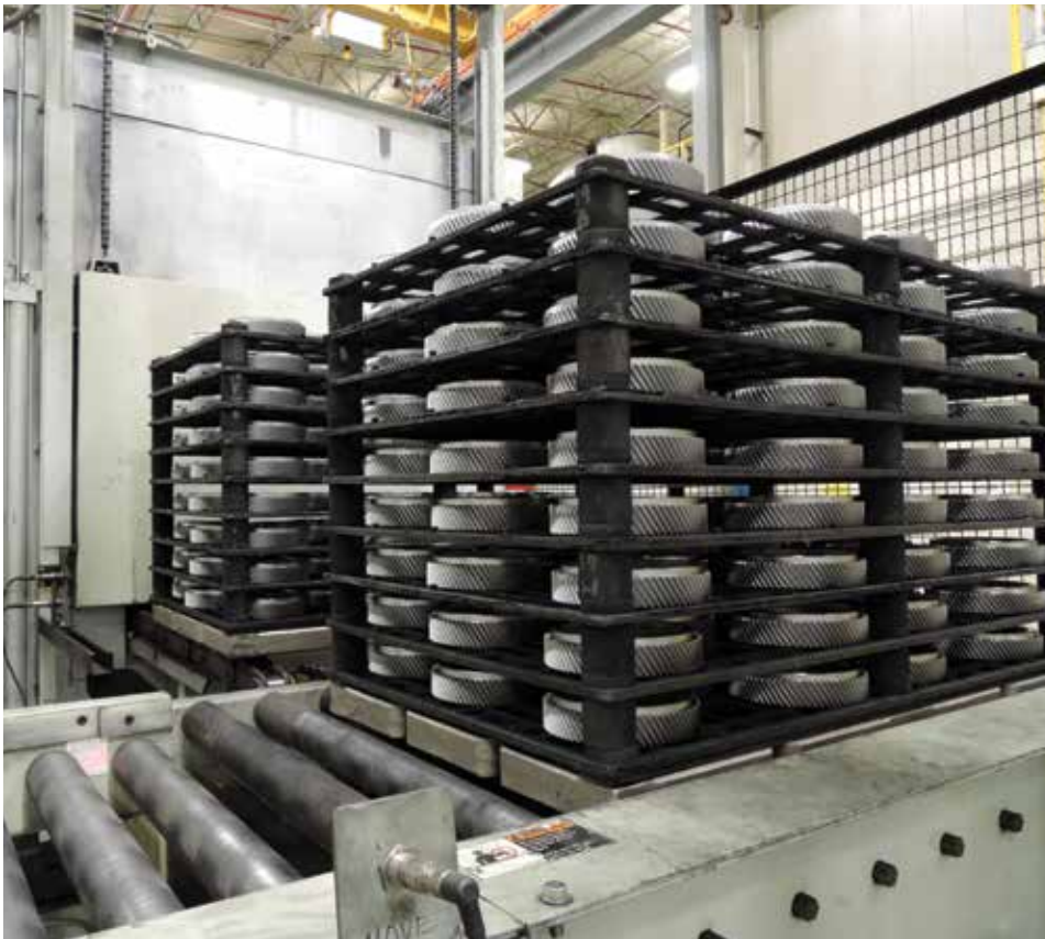
Fig 7: Typical Load of Automotive Drive Gears on UniGrid® C/C Fixturing
