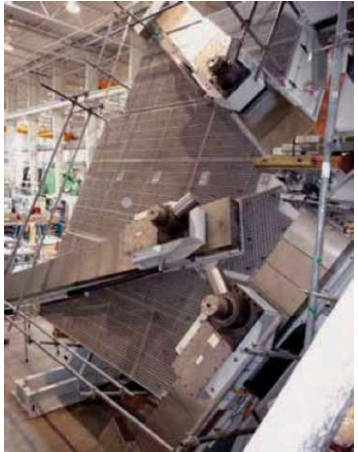
Fig. 5: SMS Elotherm Ring Hardening Machine for large bearings up to 6 m, swiveling design
