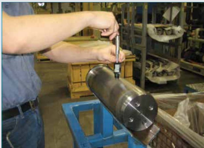
Fig. 2: Work piece firmly sitting on a solid flat surface while checking hardness.
