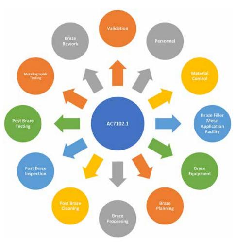
braze application and process parameters for specific part numbers. This can take many forms as suppliers typically design and use a BPS that was developed internally. The BQR qualifies general aspects of a braze based on base metal, filler metal, joint type, thermal cycle parameters, etc. This document qualifies the braze with both inspection techniques and metallurgical examination. Question 2.1 in
