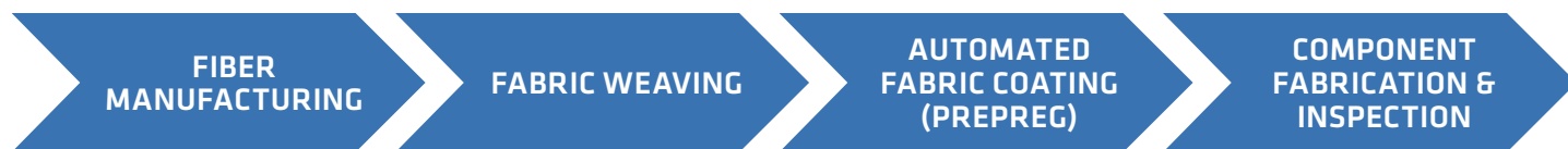
Figure 2: Typical OxOx CMC supply chain from fiber to component.
