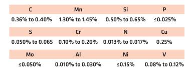
Table 1: Chemical composition as specified by the bearing manufacturer; all data points are given in weight percent.
