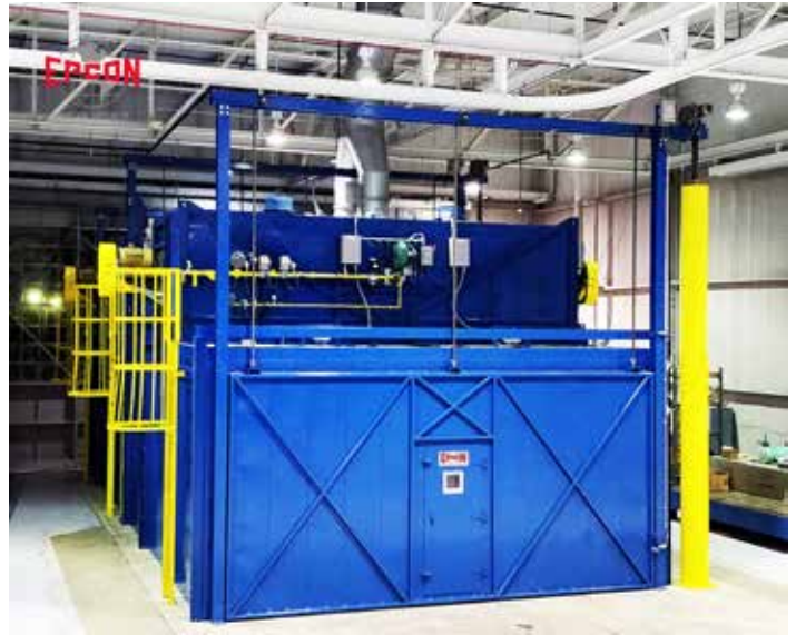
Epcor Industrial Systems' EELV curing oven and its control system are custom-designed to secure the constant quality production with monitoring where the user is notified by alarm if any of the parameters reached the critical boundary value. (Courtesy: Epcor Industrial Systems)
