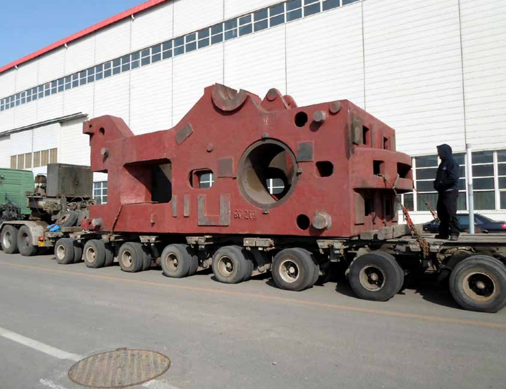
The sheer size and complexity of forging equipment means that even items such as the massive cast steel frame can take six to eight months for delivery – not including the four to six months to install all the internal parts and components. (Courtesy: Ajax-CECO)
