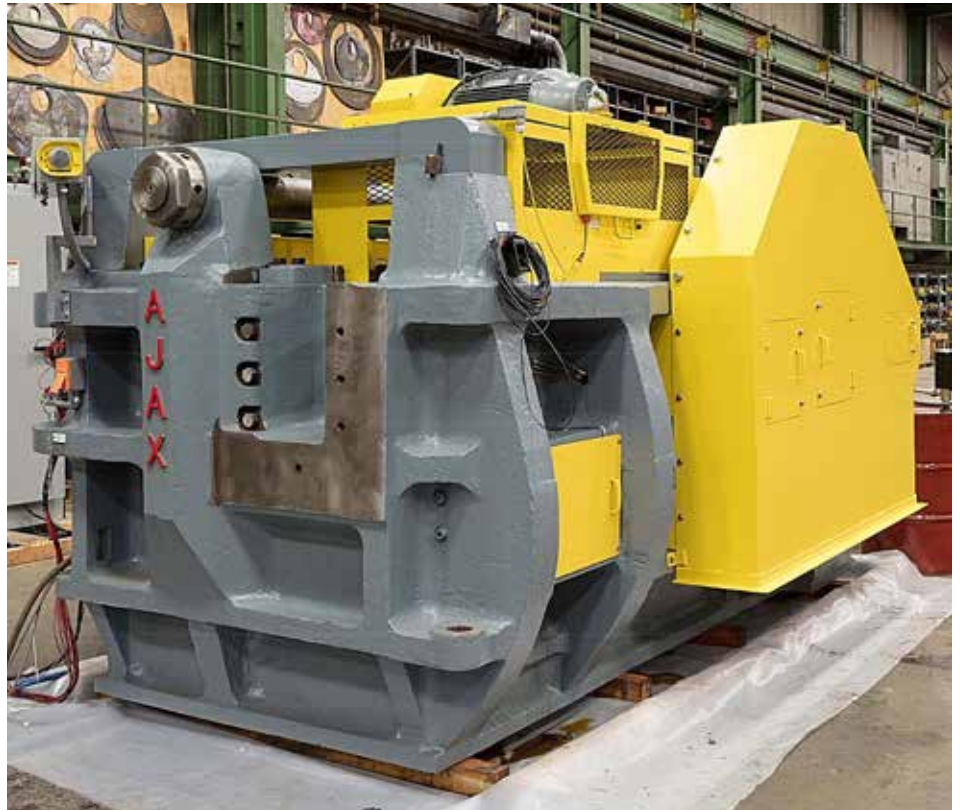
Sometimes only the cast steel frame of the forging equipment is salvageable, in which case all the internal components can be replaced in a full remanufacture of the equipment. (Courtesy: Ajax-CECO)
