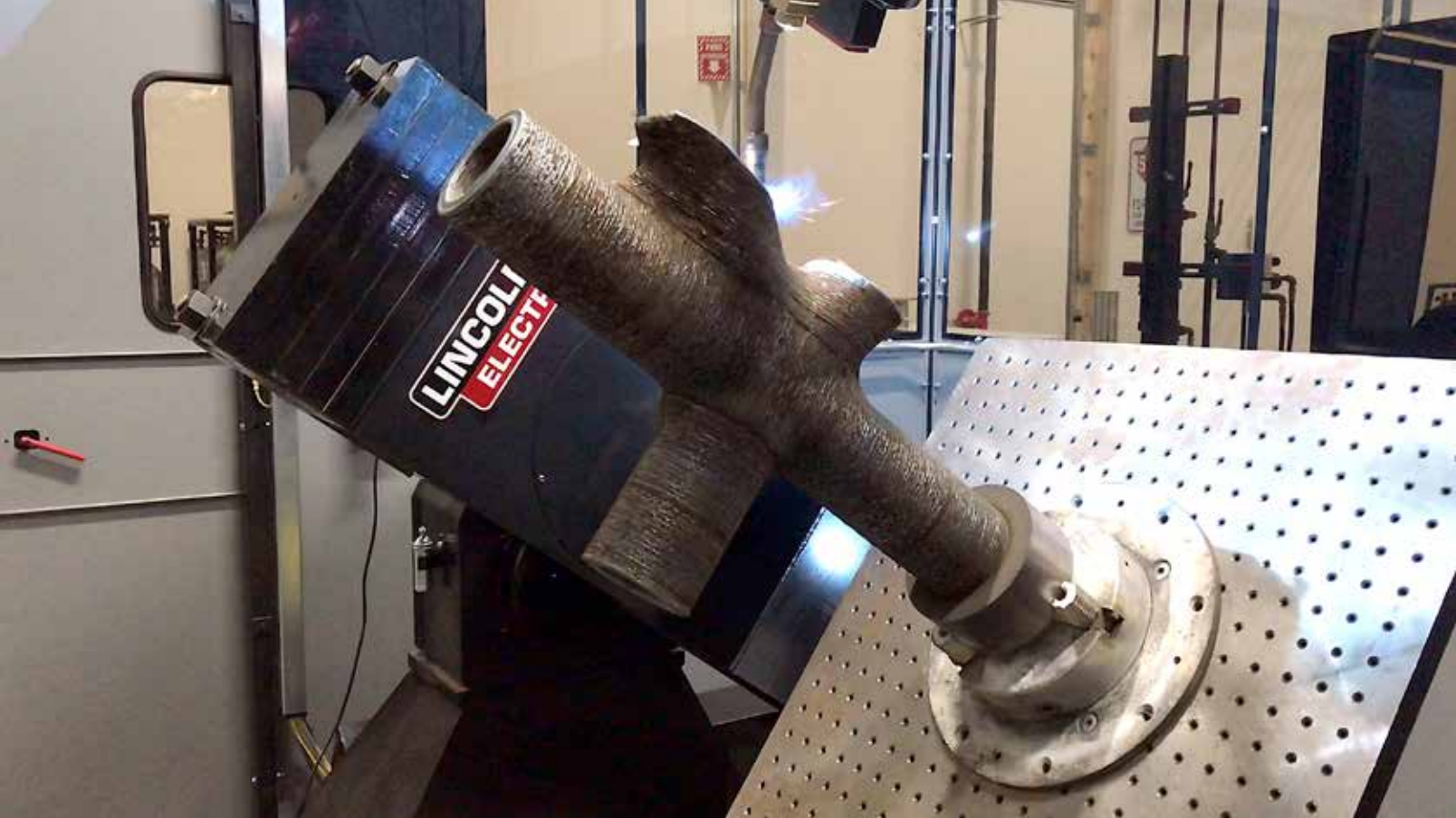
Lincoln Electric Additive Solutions' technology can 3D-print complex shapes without support structures. (Courtesy: Lincoln Electric)
