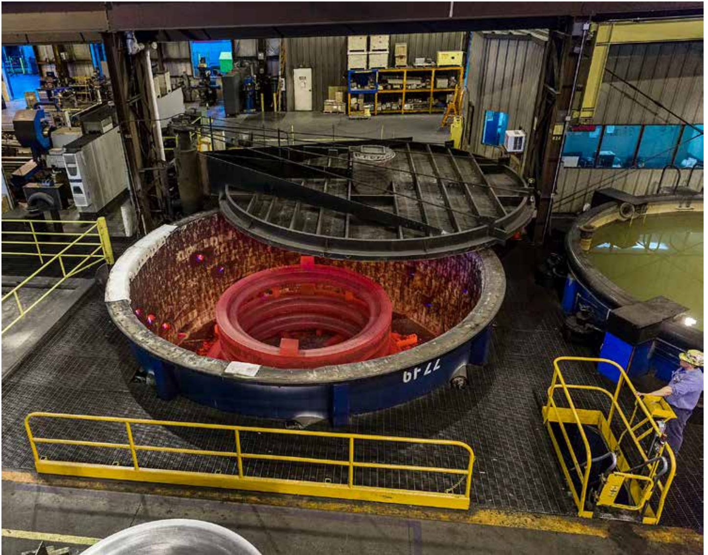
A 20-foot diameter pit furnace heats rings next to the 42,000-gallon polymer and water quench pit tank. (Courtesy: Scot Forge)
