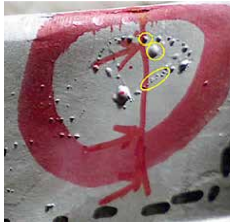
Figure 4: Blistering occurring in a 7XXX alloy.
