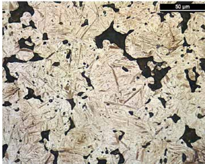
Figure 11: FL-5305 microstructure from Location C.
