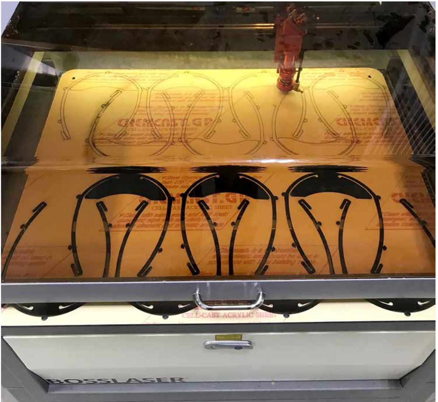
Alabama Power's Technology Applications Center uses lasers to cut the acrylic for face shields.
