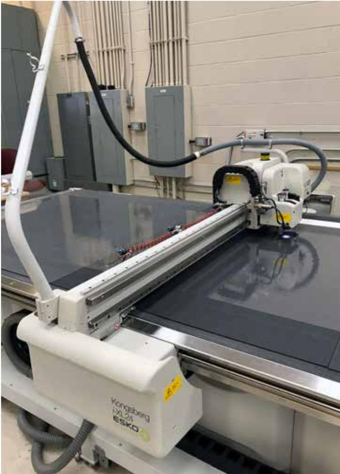
A print shop laser cuts face shields. About 100 a day can be produced this way.
