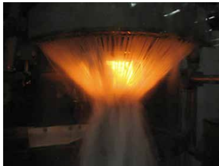
Figure 2: Blocked holes and non-uniform quenching can create soft spots. It can also increase the chance of cracking.
