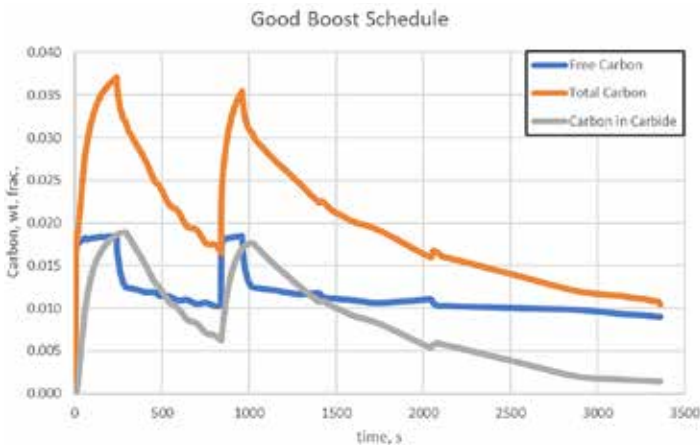
Figure 4: Properly defined boost/diffuse steps in which the carbides are mostly dissolved by the end of each diffuse step.
