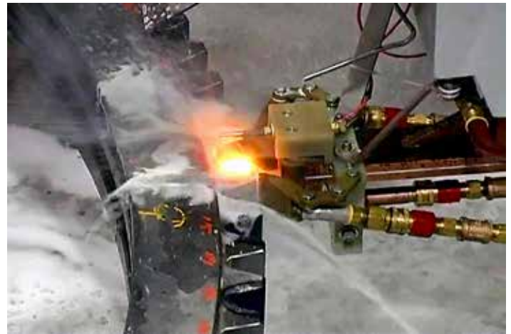
Robotic gap by gap gear scanner for the power generation industry. (Courtesy: Taylor-Winfield)
