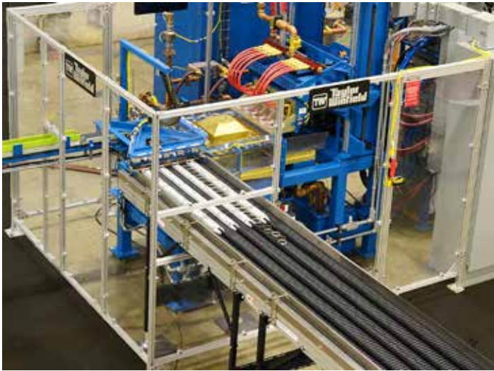
Automated high-volume induction case hardening system for small gear production. (Courtesy: Taylor-Winfield)
