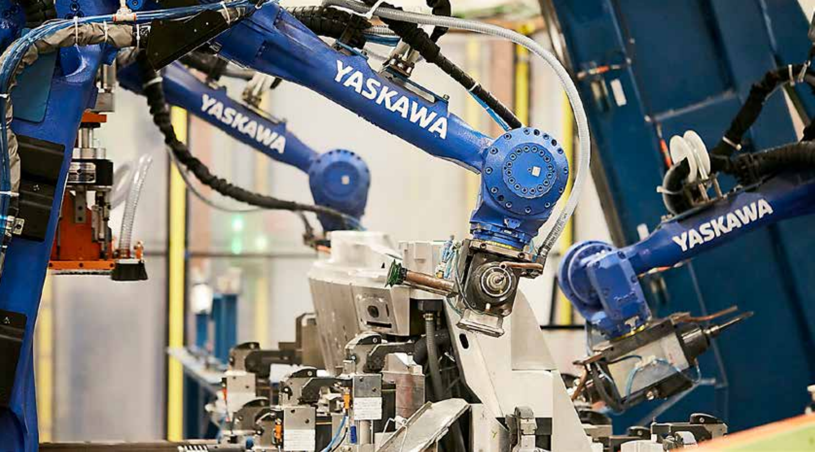
Multi-station robotic assembly system for the automotive industry. (Courtesy: Taylor-Winfield)
