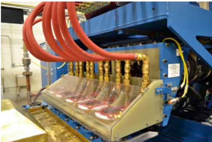
The five-lane automated system's inductor bank. (Courtesy: Taylor-Winfield)
