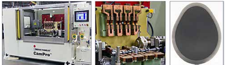
Figure 7: A CamPro® machine that uses SHarP-C™ (left), multi-lobe inductor design (center), and hardness pattern (right). (Courtesy of Inductoheat Inc., an Inductotherm Group Company)
