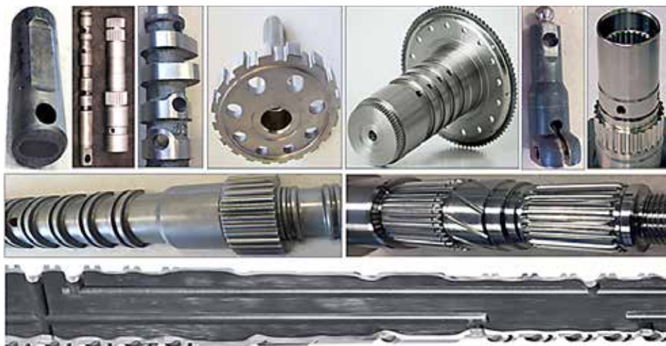
Figure 4: Examples of parts containing various holes: longitudinal (axial), transverse, and cross holes.
