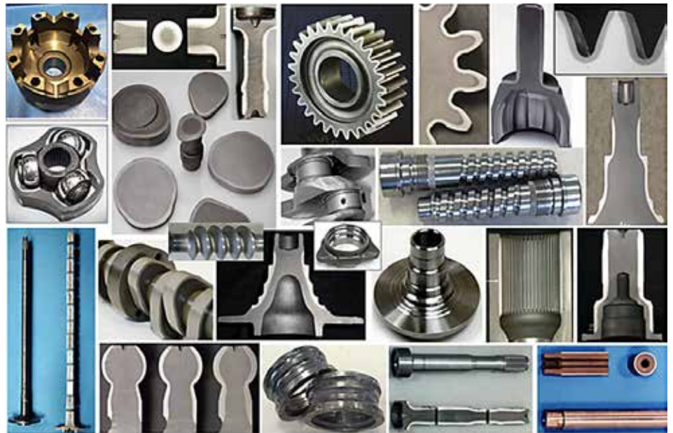
Figure 1: A small array of components that are routinely induction hardened and hardness patterns.
