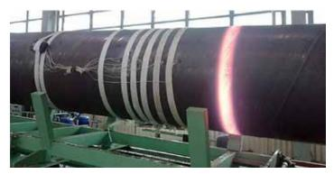
Figure 6: Experimental equipment and temperature distribution of the induction-heated steel pipe.
