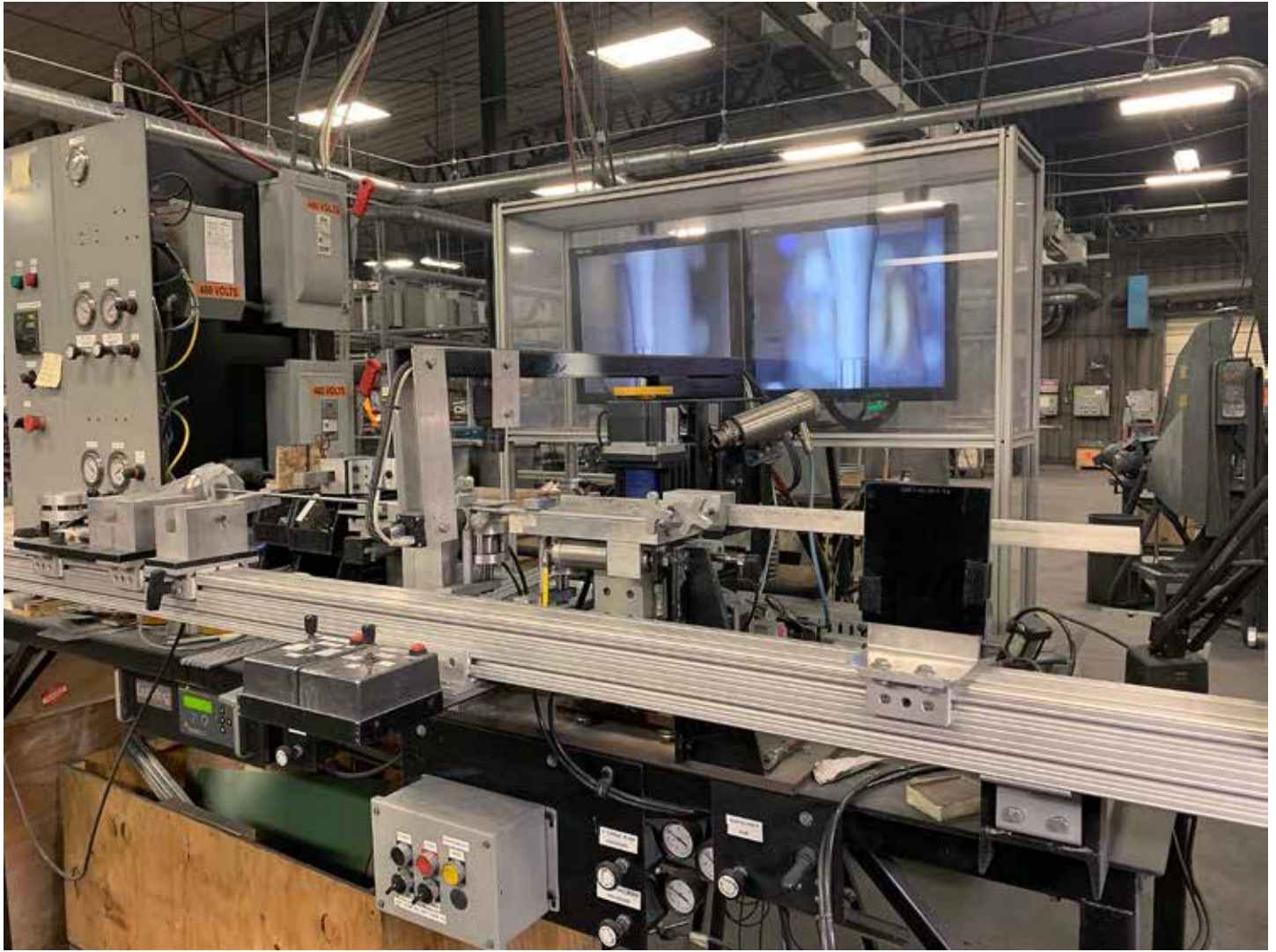
A Moly-D automatic welding machine set up with close-up video for perfect alignment of the parts to be fused.
