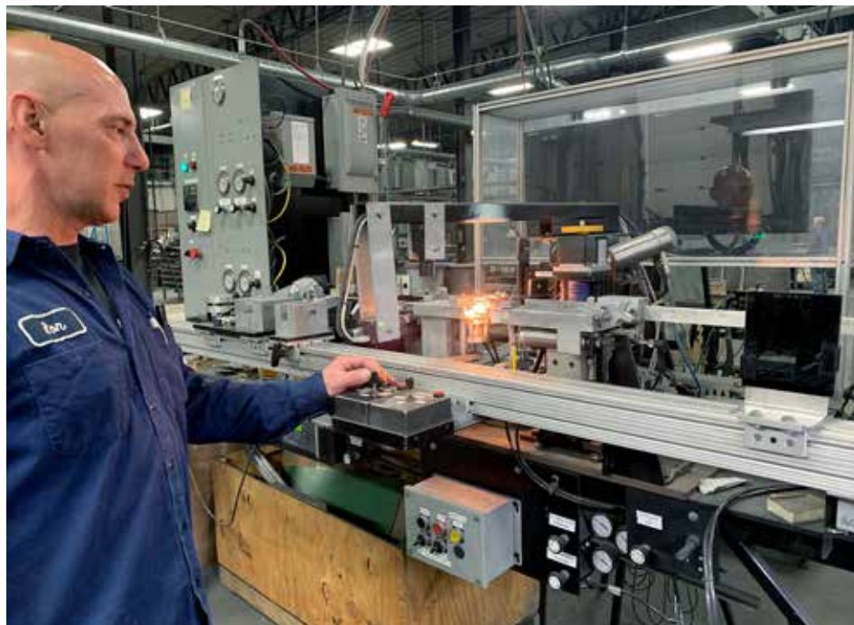
A Moly-D element being welded.
