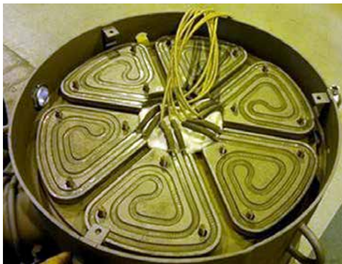
The bottom of an Agilent HS-20 diffusion pump with six Dalton Diff-Therm® 2448-10R Platen Heaters. (Courtesy: Agilent Technologies - Vacuum Products Division, Lexington, Massachusetts)
