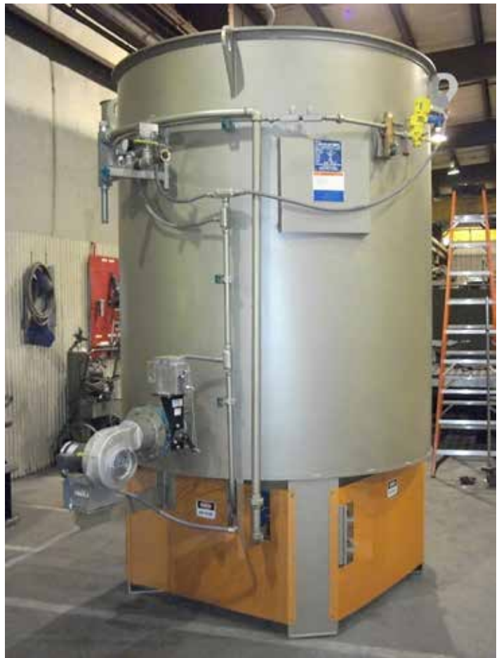
Figure 2: Steam treating with cooling blower.
