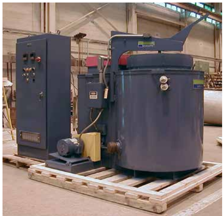
Figure 1 (A&B): Tempering furnace with cutaway view.
