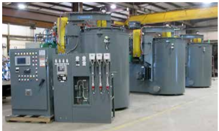
Figure 3: Gas-nitriding furnace cell.
