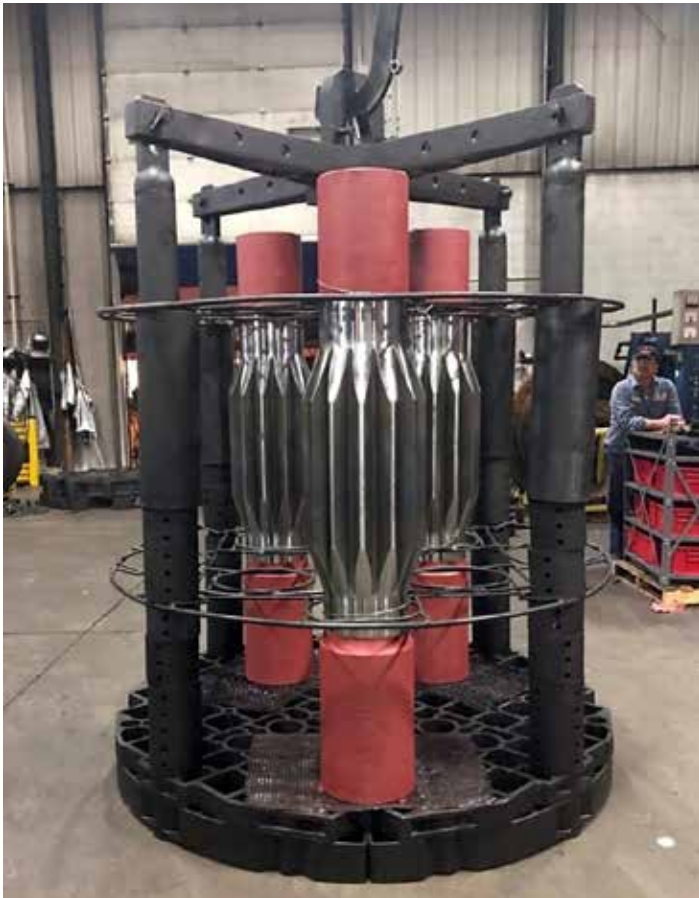
Figure 5: Typical pit carburizing load.
