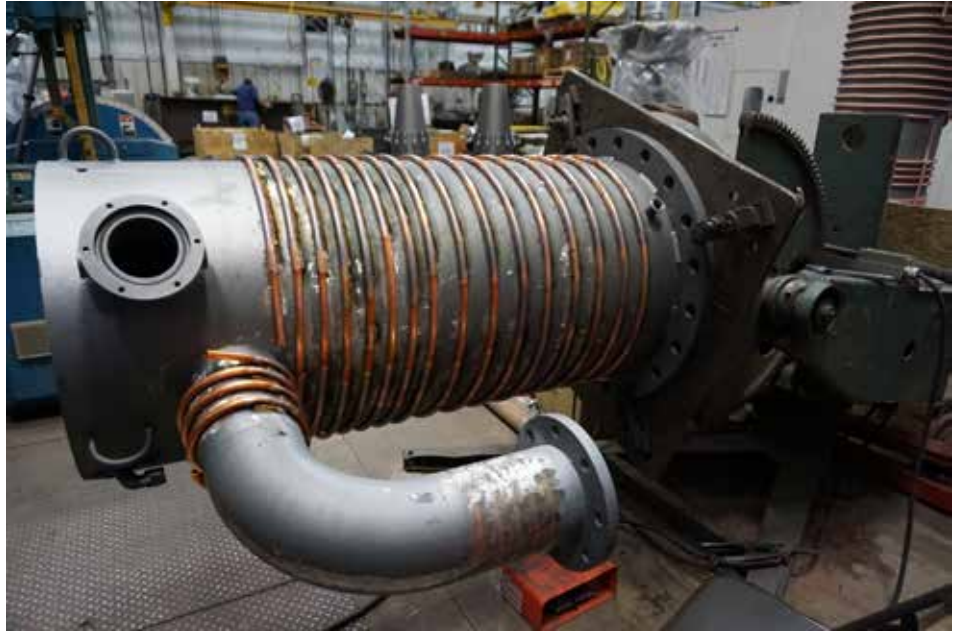
Diffusion pump receiving a new waterline tracing on the body and foreline.
