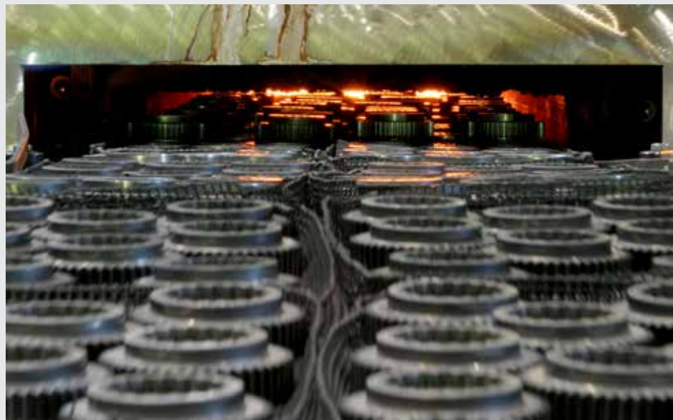
This is a 60-foot-long continuous belt furnace consisting of three zones: pre-heat 1,550°F, high heat 2,075°F, and cooling zone. In the first zone, the lubricant is removed (burnt out of) from the powder and slight particle bonding occurs; in the high heat zone, the alloying constituents, i.e. copper, nickel, molybdenum, diffuse into the iron base, and full particle bonding is achieved. Finally, the cooling chamber “cool down rate” can be varied to achieve the desired component hardness. (Courtesy: Capstan Atlantic)
