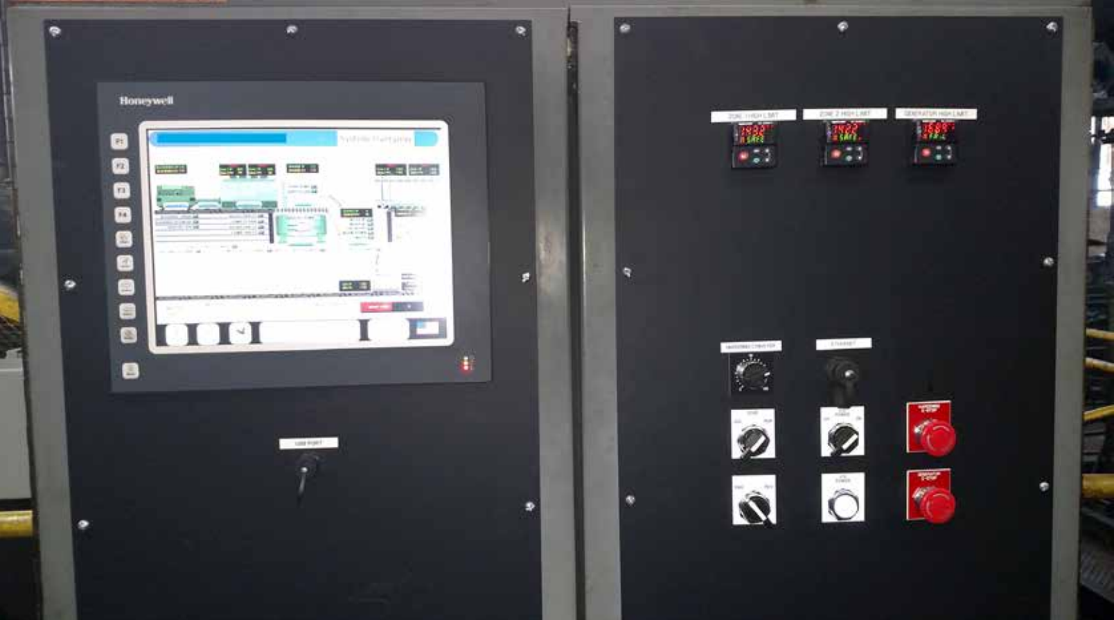
The new system includes an operator interface on the floor for ease of use, and with SpecView software tracking everything, it collects data for anything that records temperatures. (Courtesy: Conrad Kacsik)
