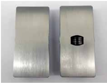
Figure 3: Artificial pore before HIP (right) and after HIP (left).
