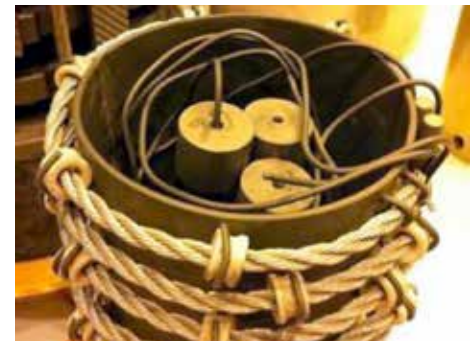
Figure 8: Set-up of samples with thermocouples in the HIP furnace.
