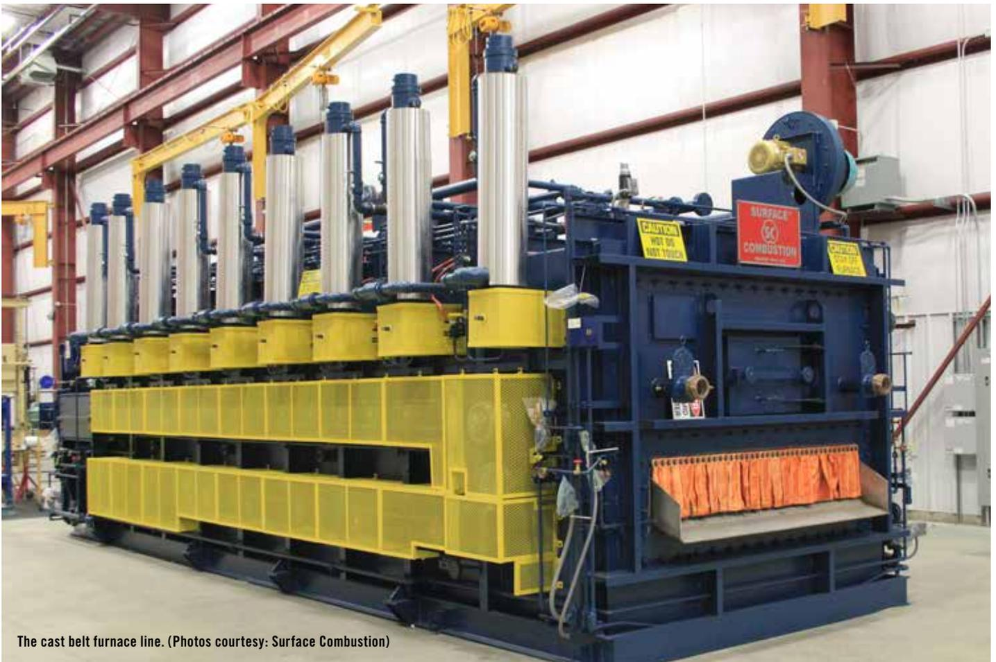
The cast belt furnace line. (Photos courtesy: Surface Combustion)
