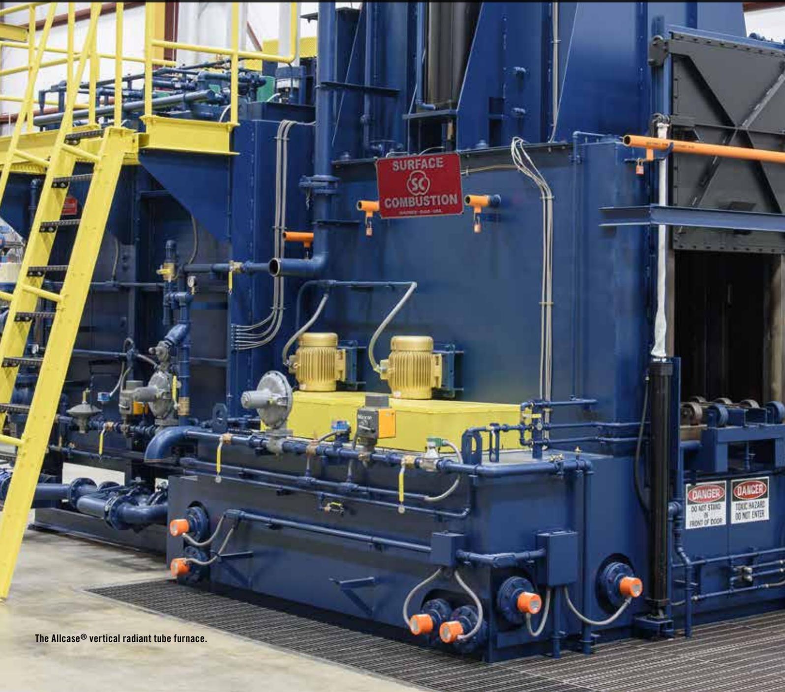
The Allcase® vertical radiant tube furnace.
