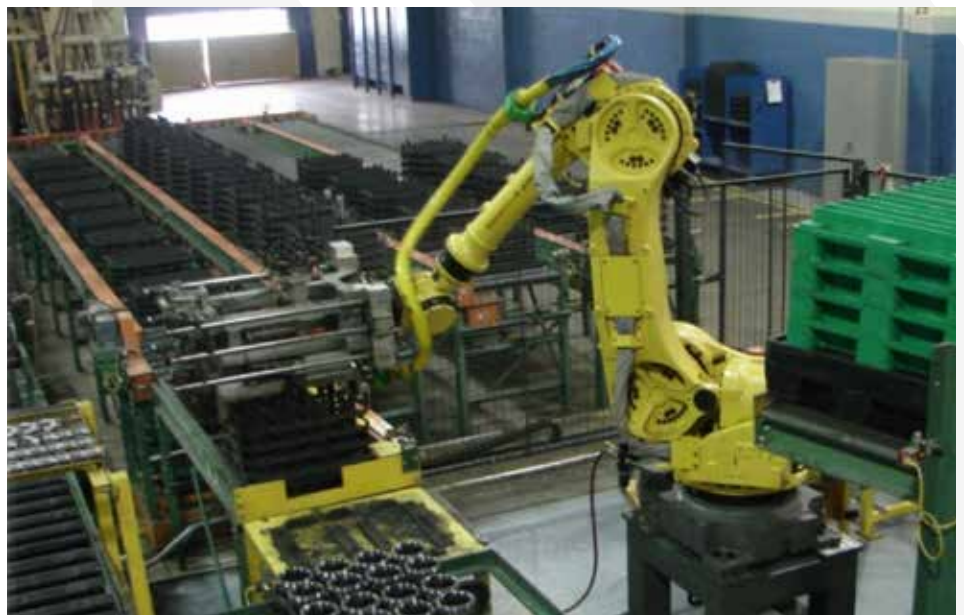
Figure 3: Robotic cell for dunnage and material handling.
