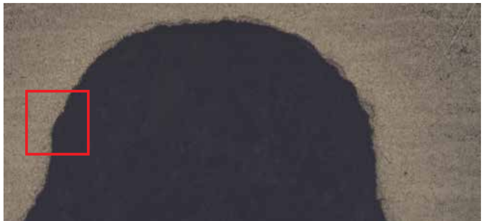
Figure 13: Root of gear and IGO test location at 60°.
