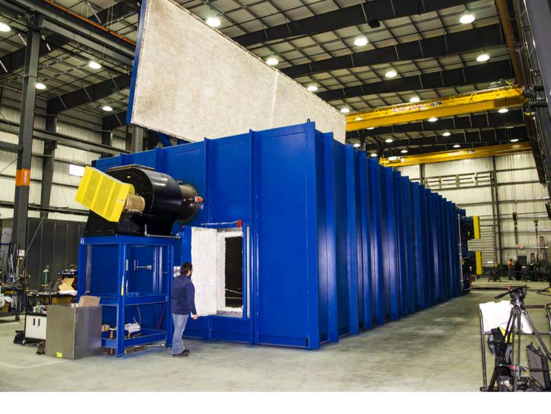
and a lot of adjusting, according to Grande. The oven had to be certified at 40 points. In order to achieve that, thermocouple probes had to be installed at every 5-foot interval in the oven to verify the temperature stayed between 1,190 degrees and 1,210 degrees Fahrenheit.
