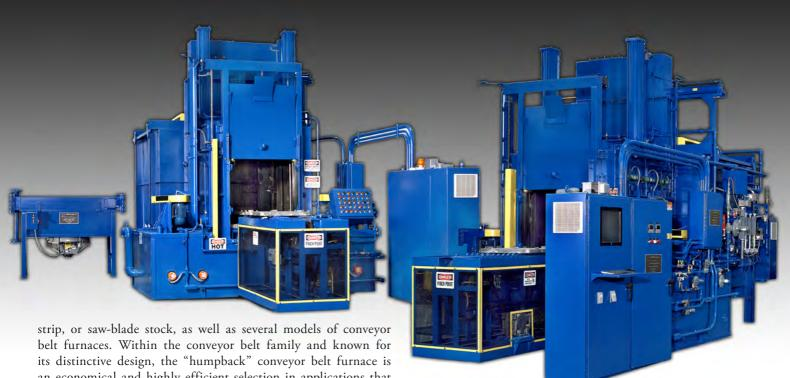
belt furnaces. Within the conveyor belt family and known for its distinctive design, the "humpback" conveyor belt furnace is an economical and highly efficient selection in applications that require extremely low dew points. Also in this family, C.I. Hayes offers the "solitaire" conveyor belt furnace with its compact design to accommodate brazing, soldering, and annealing of small pieces, such as valve assemblies and jewelry.
