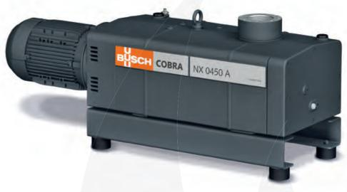
the ovens. These vacuum pumps act as the forepumps of three-stage systems incorporating booster and oil diffusion vacuum pumps. This vacuum pump arrangement can achieve ultimate pressures of up to 1x10-5 mbar in the oven process chamber. If required by the process, the pressure can be increased by introducing controlled amounts of nitrogen.
