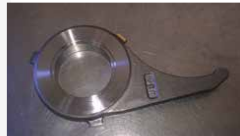
Figure 3: Lever made of 8620H material
