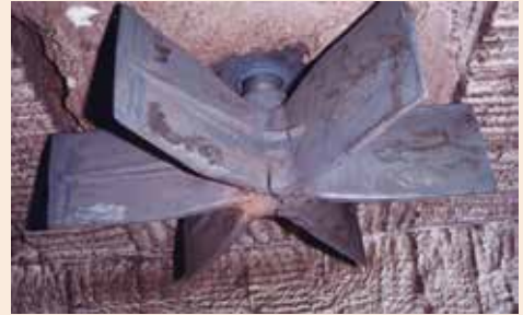
Figure 5: Thermal fatigue cracks in roof fan
