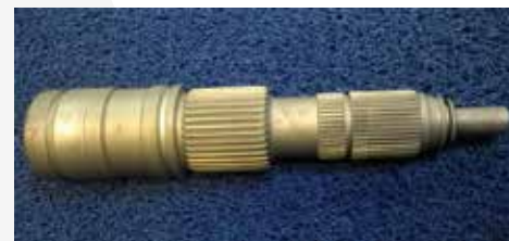
Figure 4: Shafts made of 28MnCrB7-2 material
