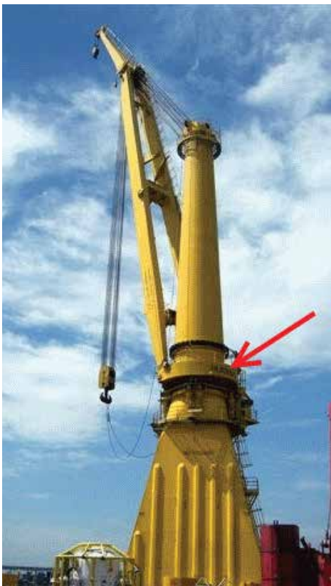
Figure 4: Crane and position of the pivot to be hardened
