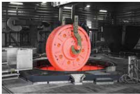
Figure 1: A 21-ton gear wheel for case hardening (source: Härtereie Reese Bochum GmbH and Horsburgh & Scott in Cleveland, Ohio)
