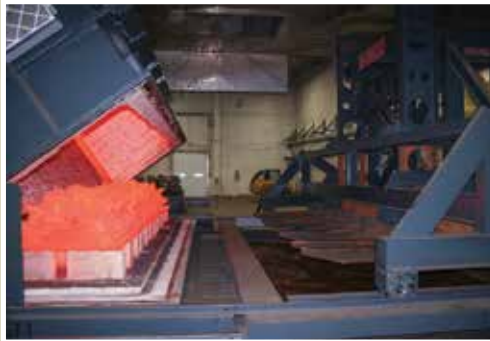
Tip-Up Furnace Capacity: 92,000 # load 33.5 feet long x 9 feet wide x 9 feet high
