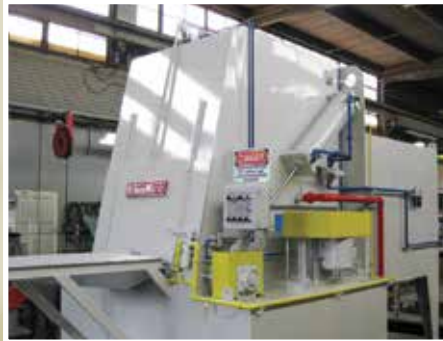
I.Q. Furnace, Capacity: 8,000 # load Tray Size: 4 feet wide x 4 feet high x 5 feet high
