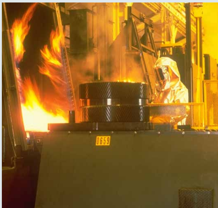
Figure 1: Atmosphere gas carburizing
