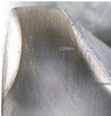
Figure 9: Conical gear wheel after hardening
