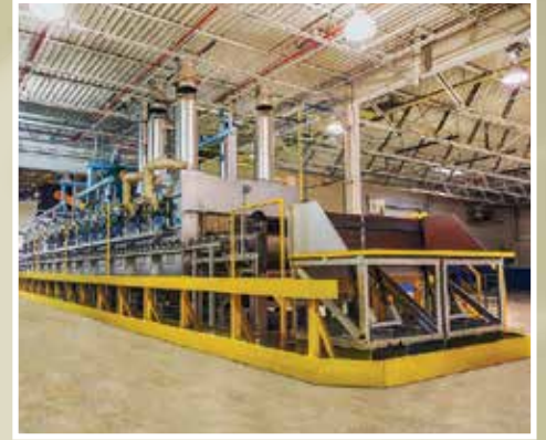
9,000#/hr Mesh-Belt Roller Hearth Annealing Furnace
