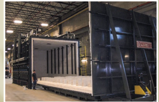
Car Bottom Furnace, Capacity: 80,000 # load 45 feet long x 14 feet wide x 14 feet high
