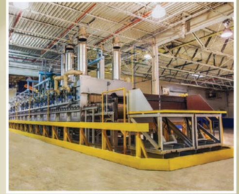
9,000#/hr Mesh-Belt Roller Hearth Annealing Furnace
