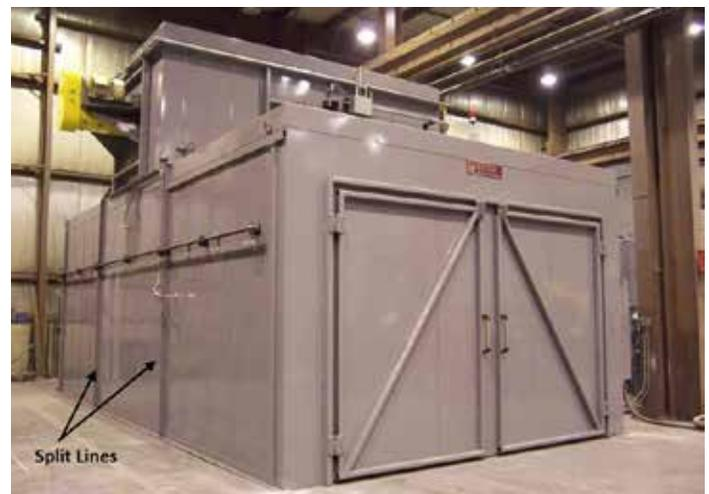
Figure 4: The body of this batch oven is designed to be split into three sections for shipment.
