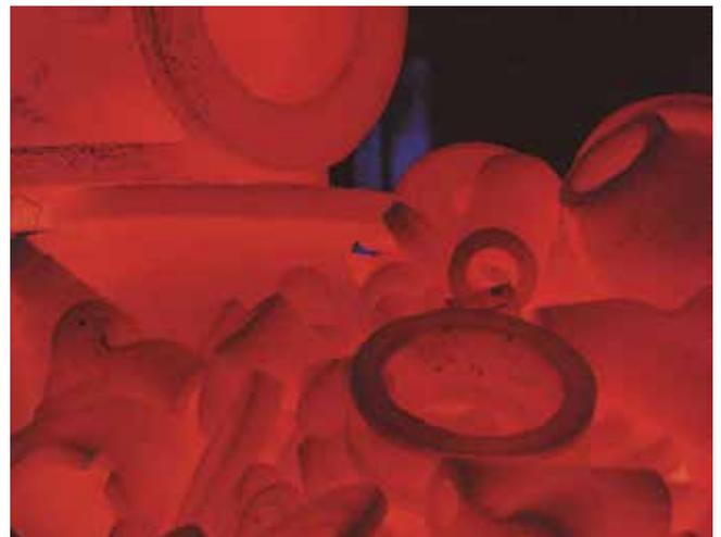
explained Vanas, Jr. "The advantage provided by oil quenching under vacuum is improved corrosion resistance and reduced crack risk for certain stainless steels."
