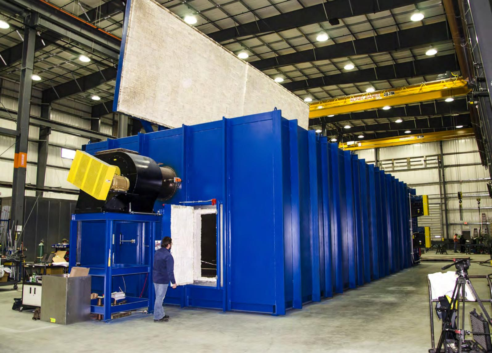
and a lot of adjusting, according to Grande. The oven had to be certified at 40 points. In order to achieve that, thermocouple probes had to be installed at every 5-foot interval in the oven to verify the temperature stayed between 1,190 degrees and 1,210 degrees Fahrenheit.
